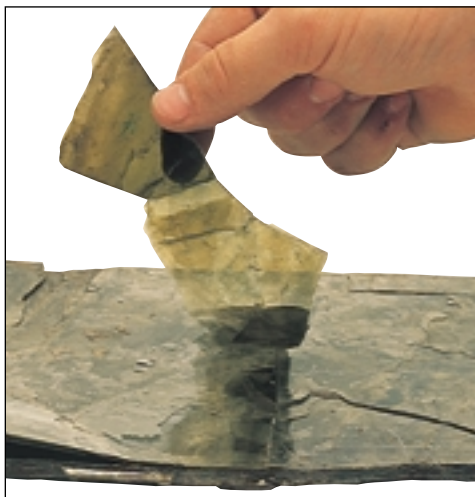
Figure 5.5 Mica is a group of minerals with a single cleavage direction that allows it to be pulled apart into sheets.
