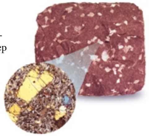
Figure 5.20 This basalt is made from magma that contained solidified crystals of minerals. The crystals can be seen clearly when a thin piece of the rock is viewed through a high-powered microscope.
