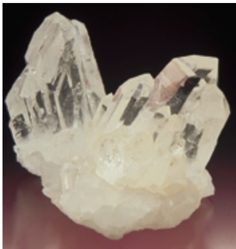
Figure 5.6 The picture above shows both the crystal faces of quartz and the fracture on the bottom of the specimen.
