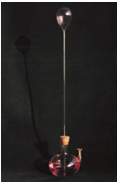
Figure 3.4A Galileo invented his air thermometer around 1600. As the air in the upper bulb cooled or warmed, a bubble of liquid moved up or down in the tube.
